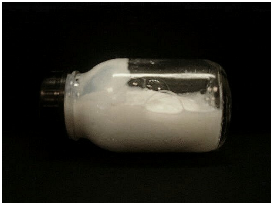
Picture 5: Syneresis in an ethylene vinyl copolymer resin binder
